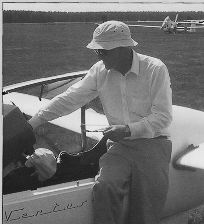
Behind Gary Ittner, a bugwiper sits in the stowed position, on the leading edge of the wing near to the fuselage.
