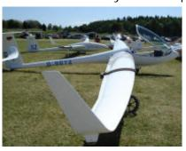
self-launch propulsion system. Large lithium-ion batteries in the wing roots drive a compact electic motor & propellor to give the Antares about 10,000' of climb on a charge. A sophisticated onboard computer system manages the engine operation, battery charging and other functions (it can give voice messages and is rumored to be capable of calling the factory if any sort of serious problem is noted). The
