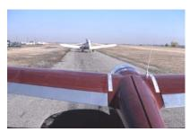
Two place trainer ready to aero tow connected by 200 feet of special rope. Image by Bill Hoadley
